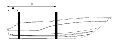
A- AFT SLING LOCATION PORT AND STARBOARD
