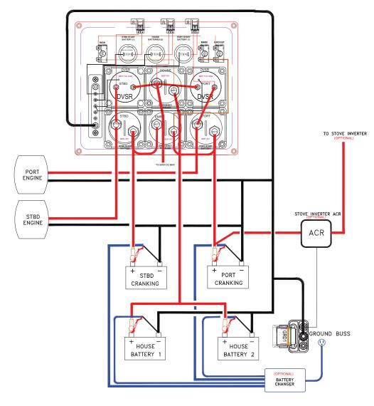
FOR NORMAL OPERATION - TURN PORT START, STBD START, AND HOUSE BATTERY SWITCHES TO THE "ON POSITION"
