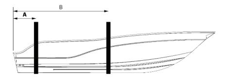
A- AFT SLING LOCATION PORT AND STARBOARD (30")
