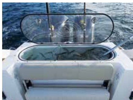
Top: Step out on one of the two swim platforms to fight a fish around the outboards. Above: The 60-gallon transom livewell is pressurized and comes with a divider.
